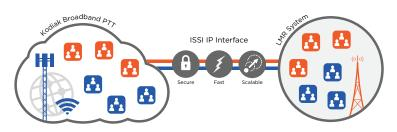
The P25 Inter-RF Subsystem Interface (ISSI) standardizes the messaging used for voice and data transport between P25 networks, making interoperable communication between multiple systems possible, even if they are using different frequency bands. ISSI also provides a common meeting place for P25 RF Sub-systems and broadband push-to-talk (PTT) networks, providing interoperable communication without the need for gateways, donor radios, and donor phones.
